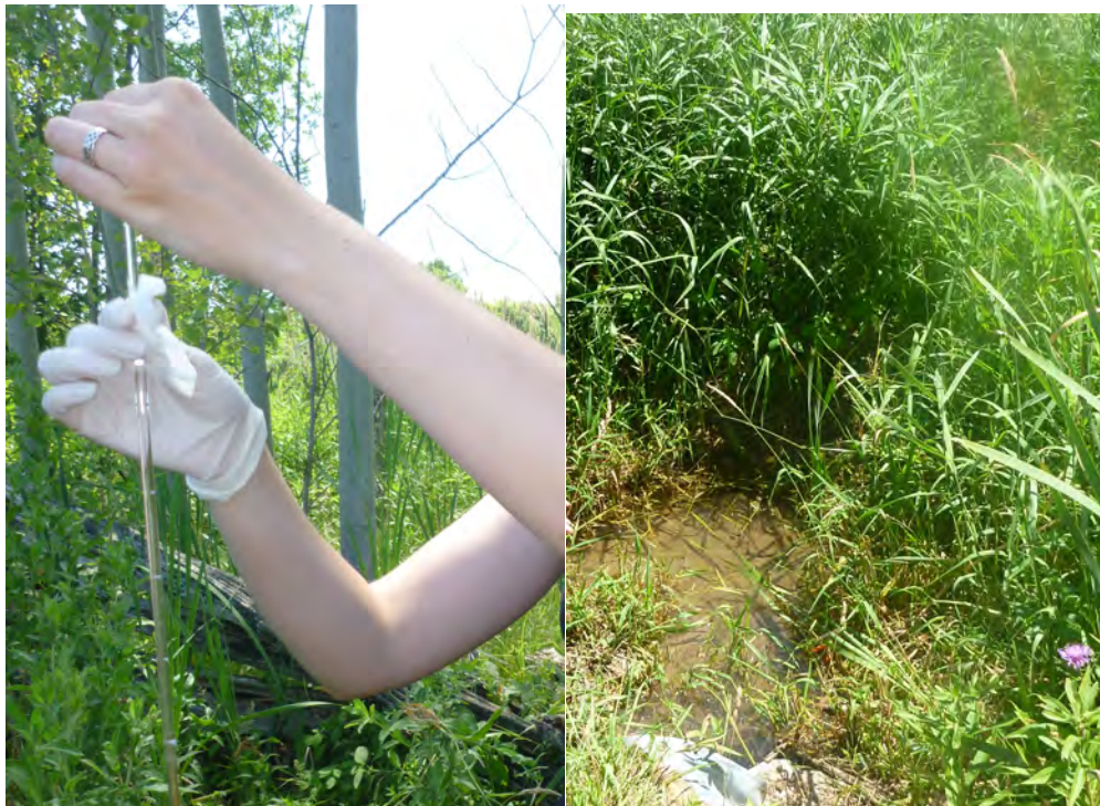
Photo 6: Photo of an acrylic rod (left panel) being prepared to be inserted into a stream (right panel).
